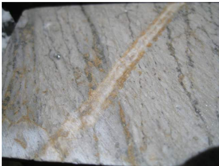
Figure 7.15 Quartz-alunite (?) veins cutting quartz-pyrite veins. Drill hole SLP-009-01, 51.4 m; photo by the author, 2011.
