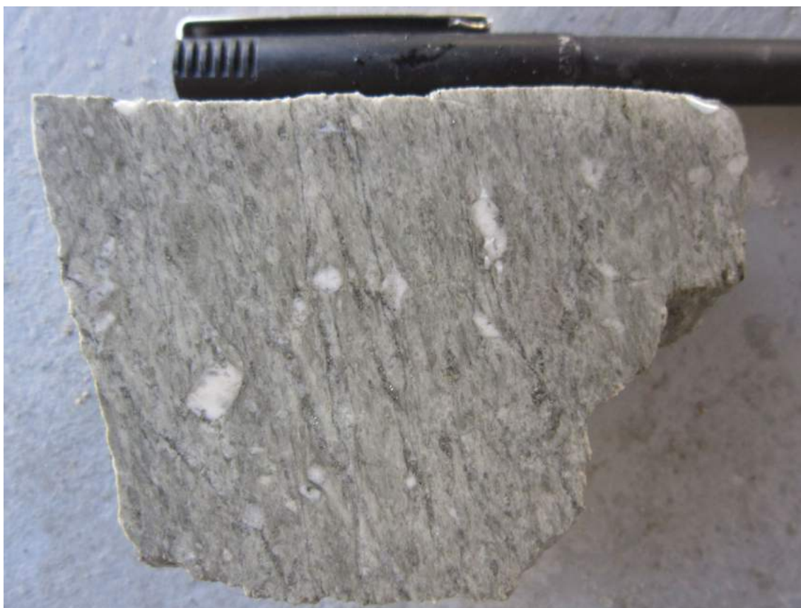
Figure 7.10 Compositional layering, fiamme, and welded textures in rhyolite. Drill hole SGL-11-02, 9.1 m.
