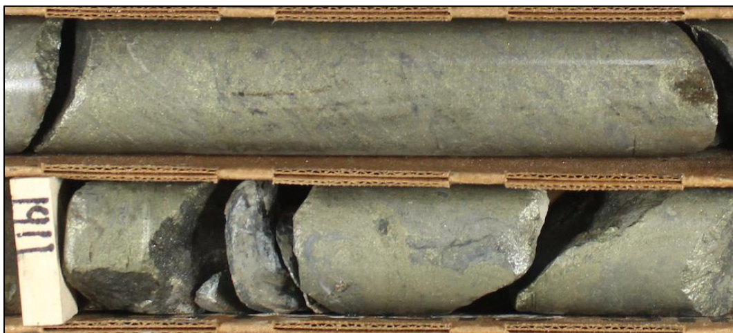
Figure 7-10 Massive Chalcopyrite in Drill Core from a 1.2-M Sample Grading 9.8% Cu, 6.1 G/T Au (Drill Hole KM-21-26, 581.6-582.8 M) (Smith, 2024)
