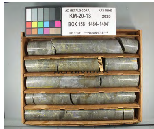
Chalcopyrite and sphalerite mineralization
